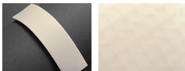
Versico VersiWeld – 60 Weeks (No Failure)
