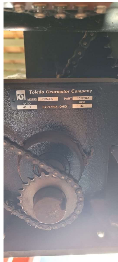
Photo B-3: Gear reducer nameplate (Toledo Gearmotor C55-ES)
